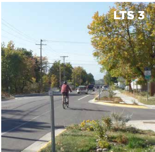
Bike lanes where traffic speeds and volumes are higher and on-street parking is present can be more stressful and may only be utilized by more experienced bicyclists.
