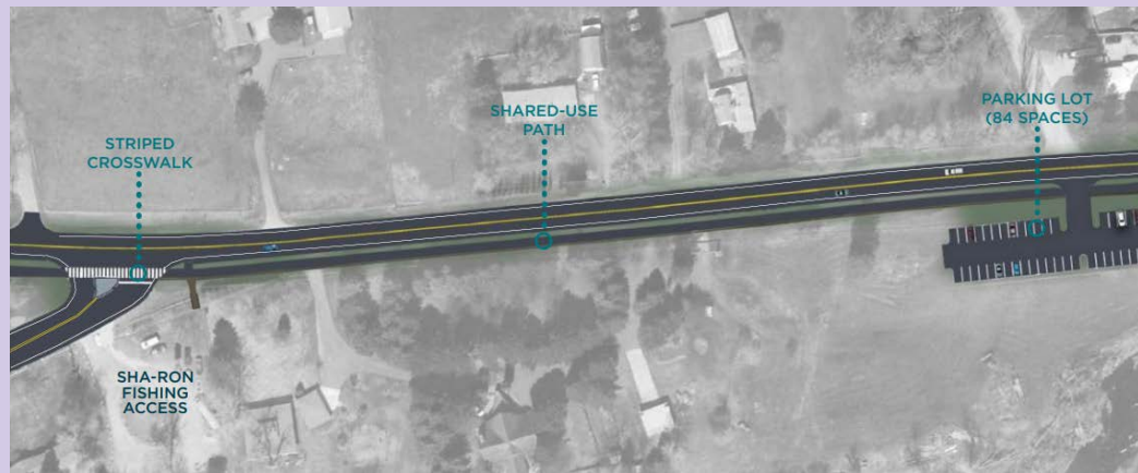
Preferred Highway 200 alternative includes a new parking lot within MDT right-of-way and a shared-use path connection to Sha-Ron fishing access
